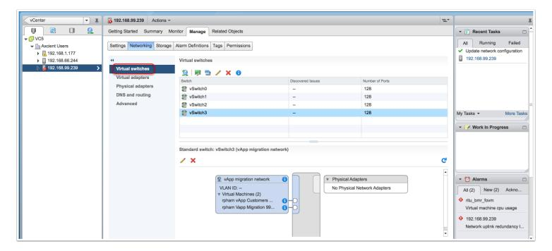
The "Virtual switches" pane should show that the two virtual machines are connected to each other.
