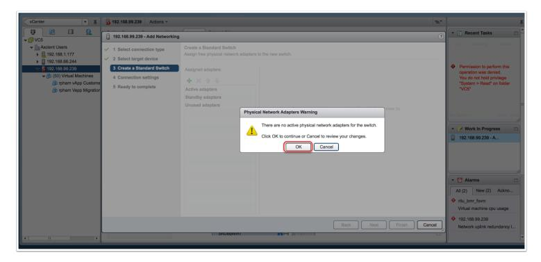
Click "OK" when the warning window displays. Since two virtual appliances are going to be connected on the same switch - no physical NIC is needed.
