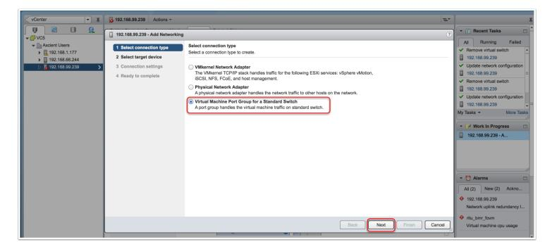
Select the connection type to be "Virtual Machine Port Group for a Standard Switch", and then select the "Next" button.
