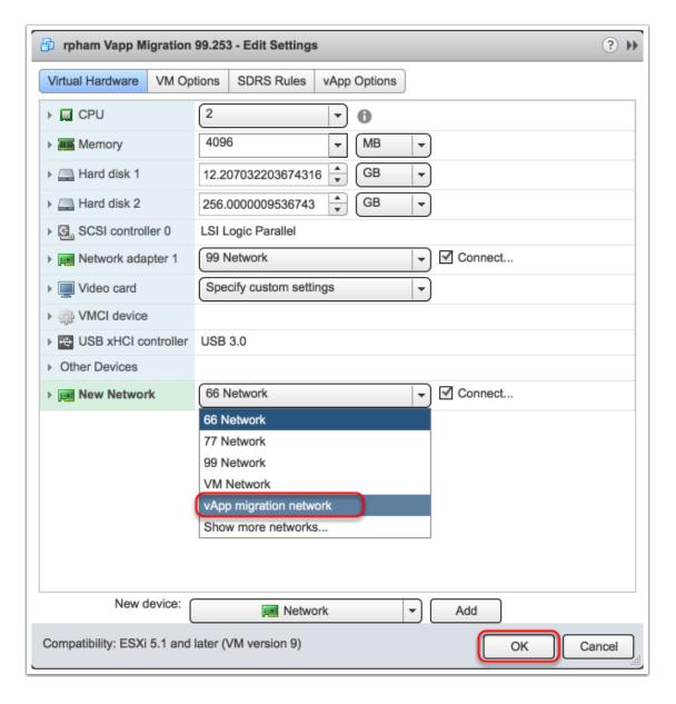
The new NIC will appear on the left side of the settings window with a dropdown next to it. Through the dropdown select the vSwitch (based on the label that you previously gave it). Then select the "OK" button.
