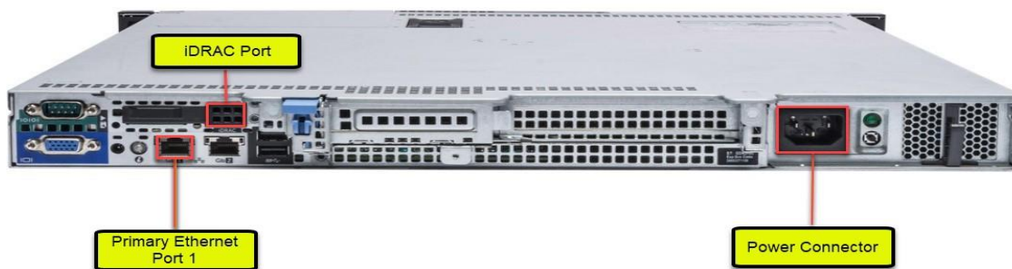
Figure 2 - Back view of the 1U appliance
