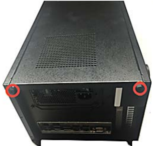
Lid access points are highlighted in this illustration in red:
